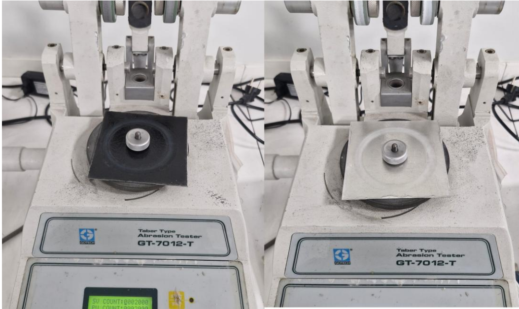
Figure 1. UPCB0 and UPCB10 composite specimens mounted on the Taber abrasion tester after the abrasion test
