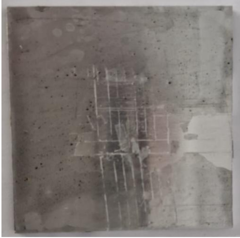
Figure 5. Photograph of UPCB0 without DPGDA specimen after the cross-cut adhesion test
